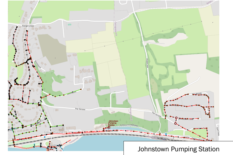
Figure 6.5 – Existing Wastewater Drainage Network
