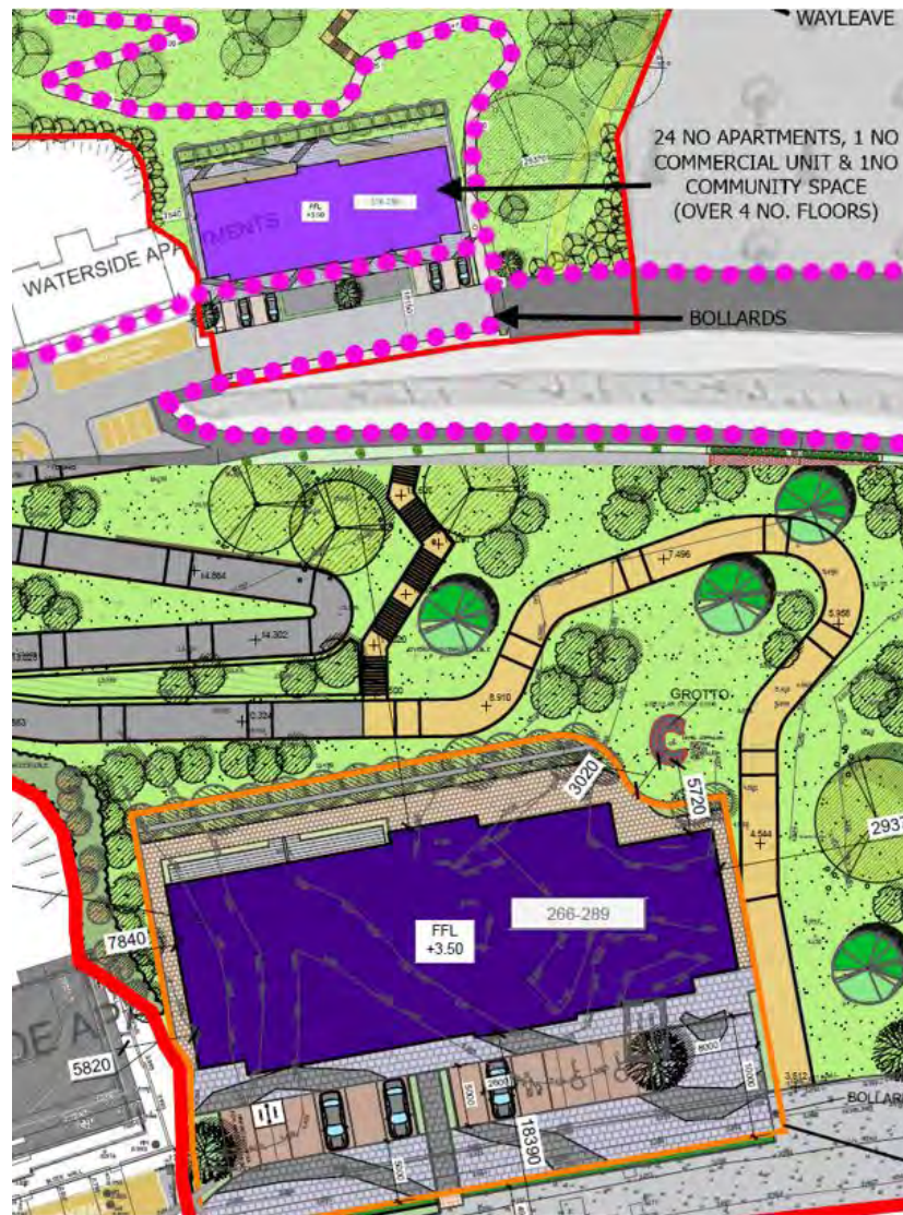
Figure 3.34 Comparison of Alternative D (top image) and Alternative E (bottom image) reflecting the evolution of the footprint of the southern apartment building, increasing separation distances to the existing grotto.
