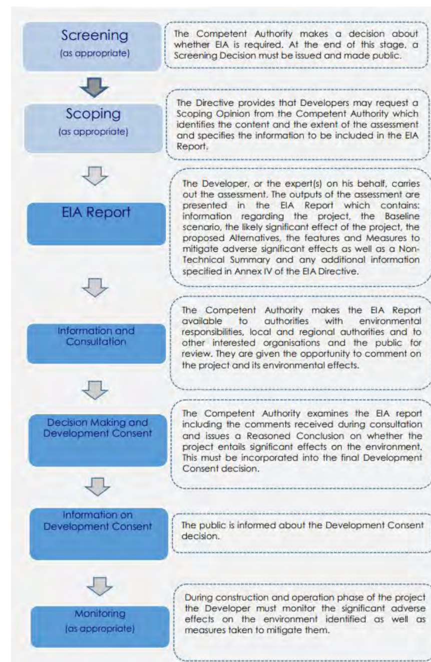
Figure 1.1 - EIA Process (Source: Page 12 of Preparation of guidance documents for the implementation of EIA Directive (Directive 2011/92/EU as amended by 2014/52/EU).
